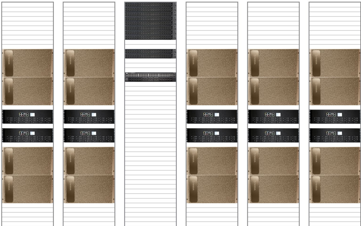
Figure 2. DGX A100 scalable unit
