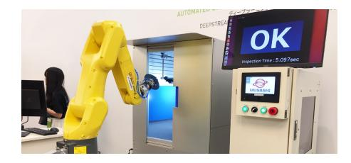
robot arm. Good parts are placed in the next stage of manufacturing, while faulty parts are rejected.
